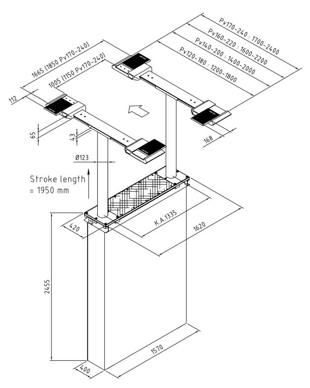
Dimension sketch incl. specification of level for drive-over height.
